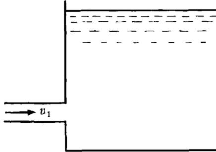
Fig. 7.8 Outlet of pipe line
