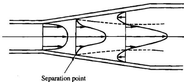
Fig. 7.15 Velocity distribution in a divergent pipe
