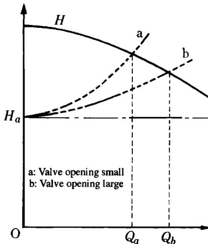
Fig. 7.26 Total head and load curve of pump
