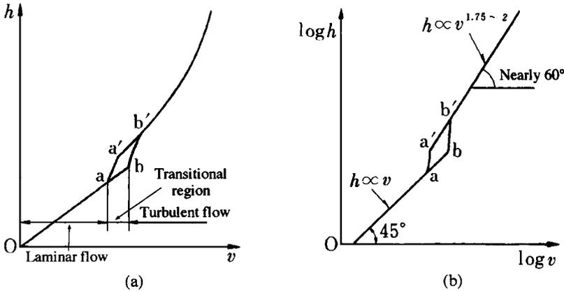
Fig. 7.3 Relationship between flow velocity and loss head
